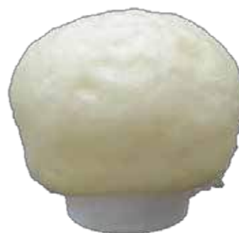
Fig. 7 : Foaming of PU Resin after exposure to water
