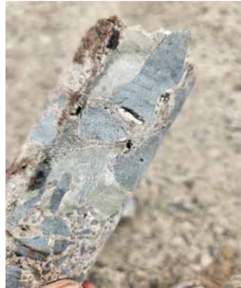
Fig 5 & 6 : Traces of new grout material in concrete cores extracted
