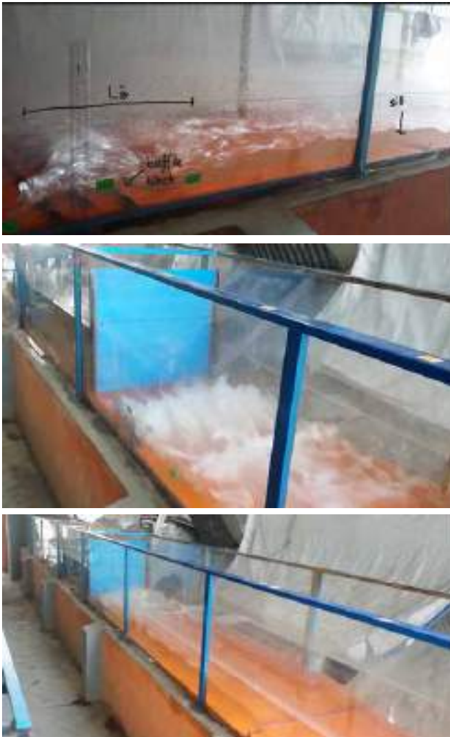
Fig. 5 : Hydraulic jump and length of jump in front of the sluice gate (Source: Sunik, 2019)
