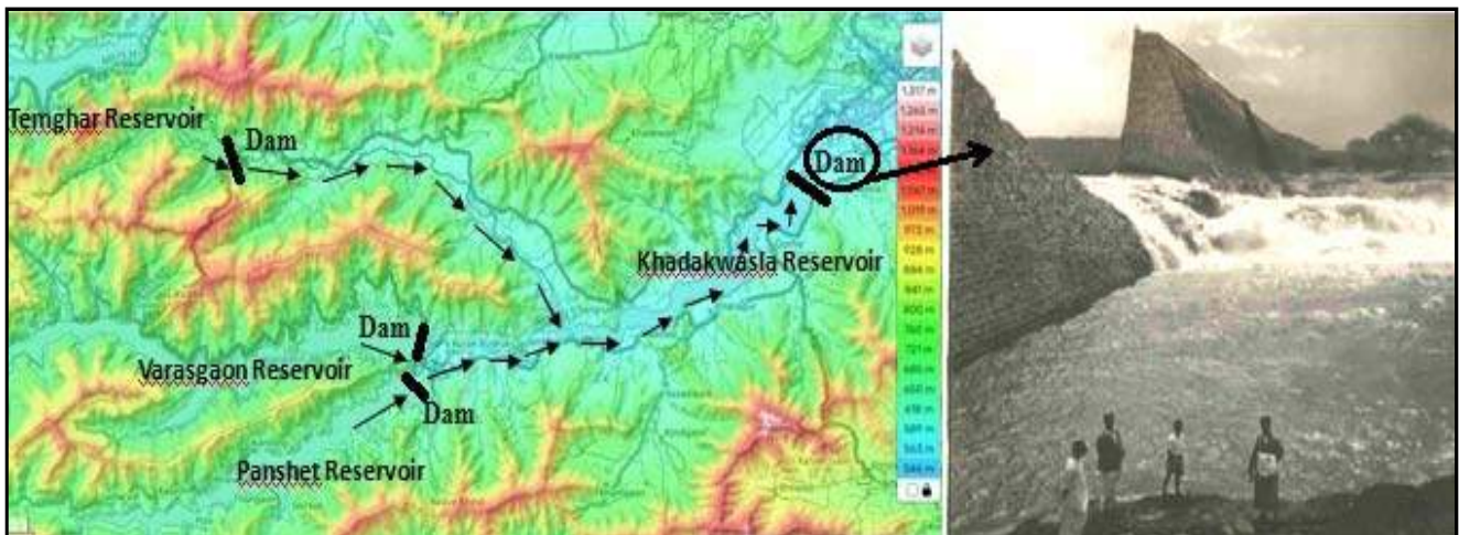
Fig. 6 : Failure of Khadakwasla Dam due to cascading impact of flood
