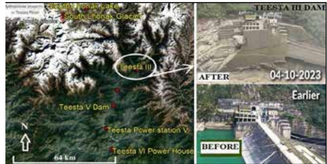
Fig. 3 : Failure of Teesta III H.E. Dam caused by GLOF
