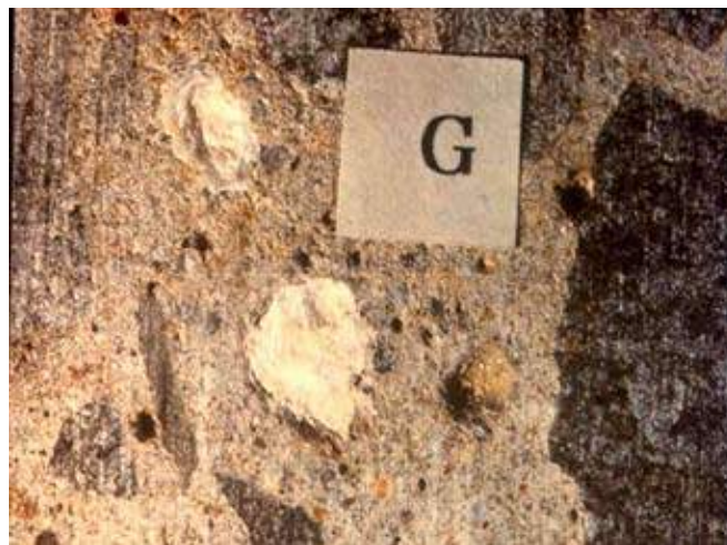
Figure 1 : Alkali silica gel inside the concrete
