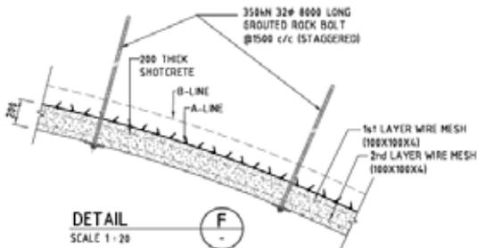
Fig. 9 : Typical support system for Fair rock (PQM+PQT)
