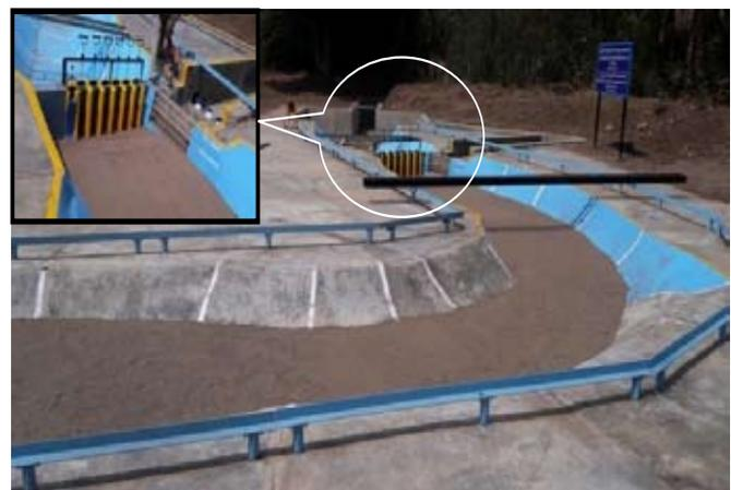
Fig. 4 : View of model showing sedimentation in reservoir as per profile-I
