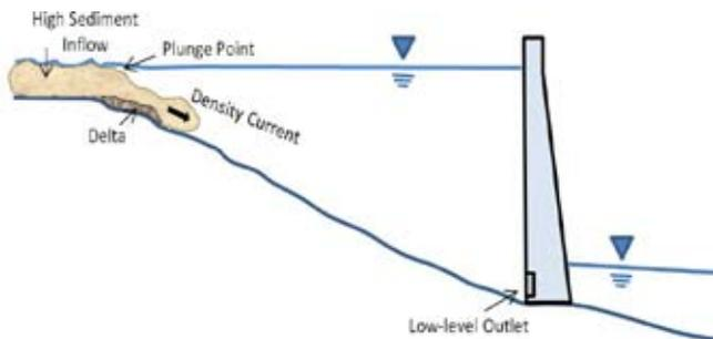
**Fig. 5 :** Density current along longitudinal reservoir profile
