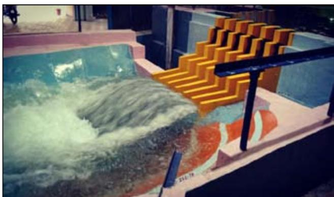
**Photo 11** : Performance of energy dissipator for the discharge of 13000 m<sup>3</sup>/s
