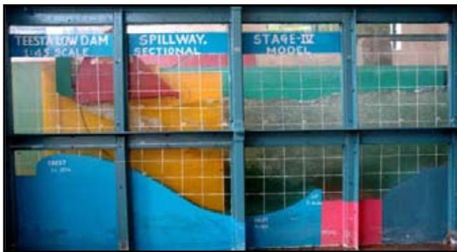
**Photo 12** : Performance of solid roller bucket for gated operation of spillway for the discharge of  $15400 \text{ m}^3/\text{s}$
