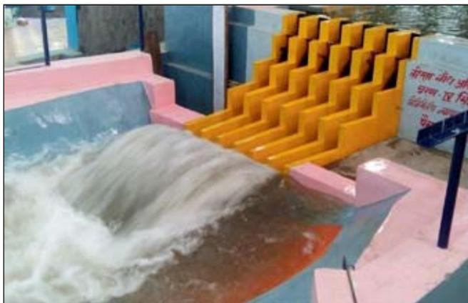
Photo 3 : Performance of energy dissipator for the discharge of 13000 m<sup>3</sup>/s
