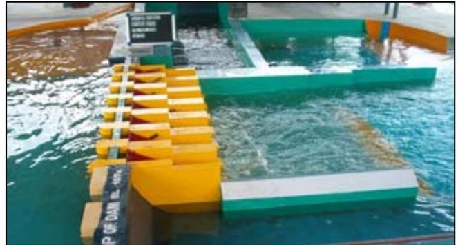
**Photo 14** : Performance of stilling basin for gated operation of spillway for the discharge of  $7700 \text{ m}^3/\text{s}$
