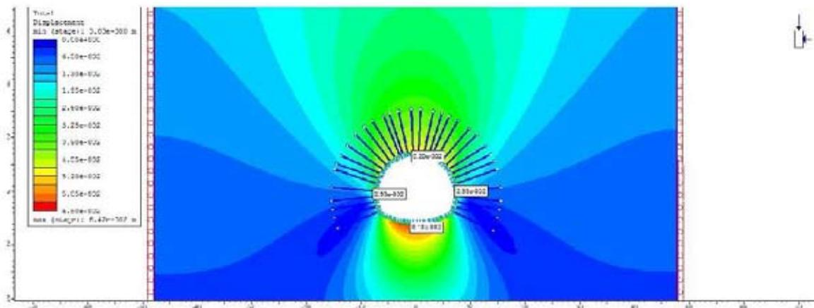
**Figure 3 :** Total displacement after complete excavation of TBM Adit.
