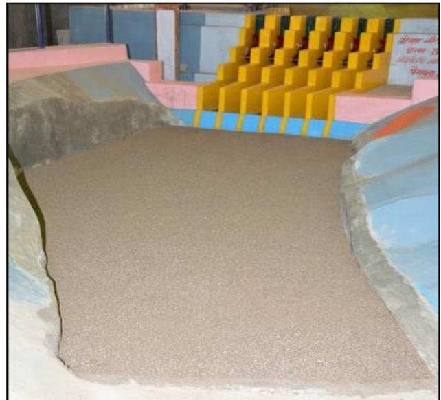
**Photo 6 :** River bed (scour pit) with erodible bed material in model
