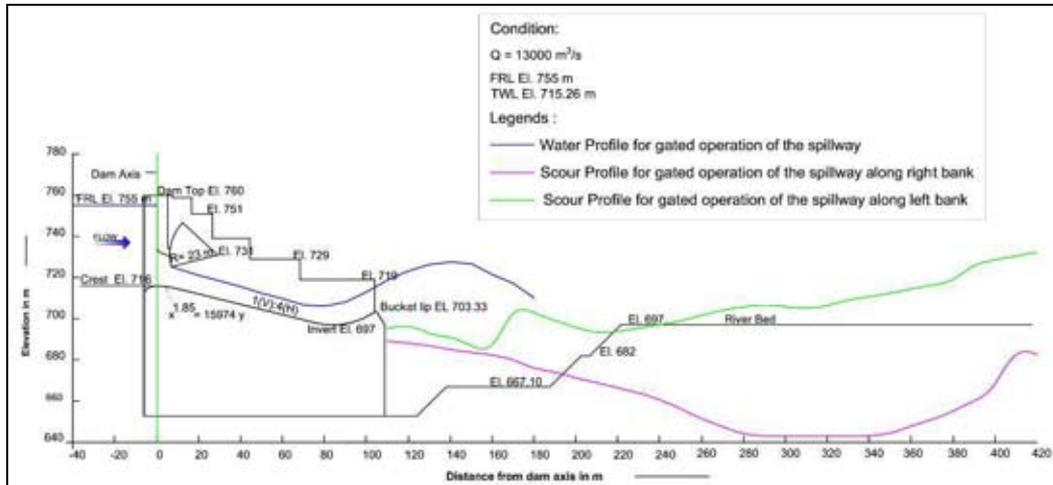
**Fig. 3 :** Water and scour profile for gated operation of the spillway
