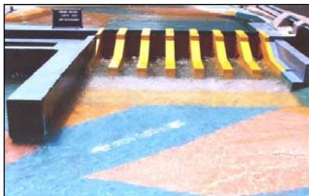
Photo 19 : Performance of stilling basin for the discharge of 5215 m<sup>3</sup>/s for gated operation of spillway
