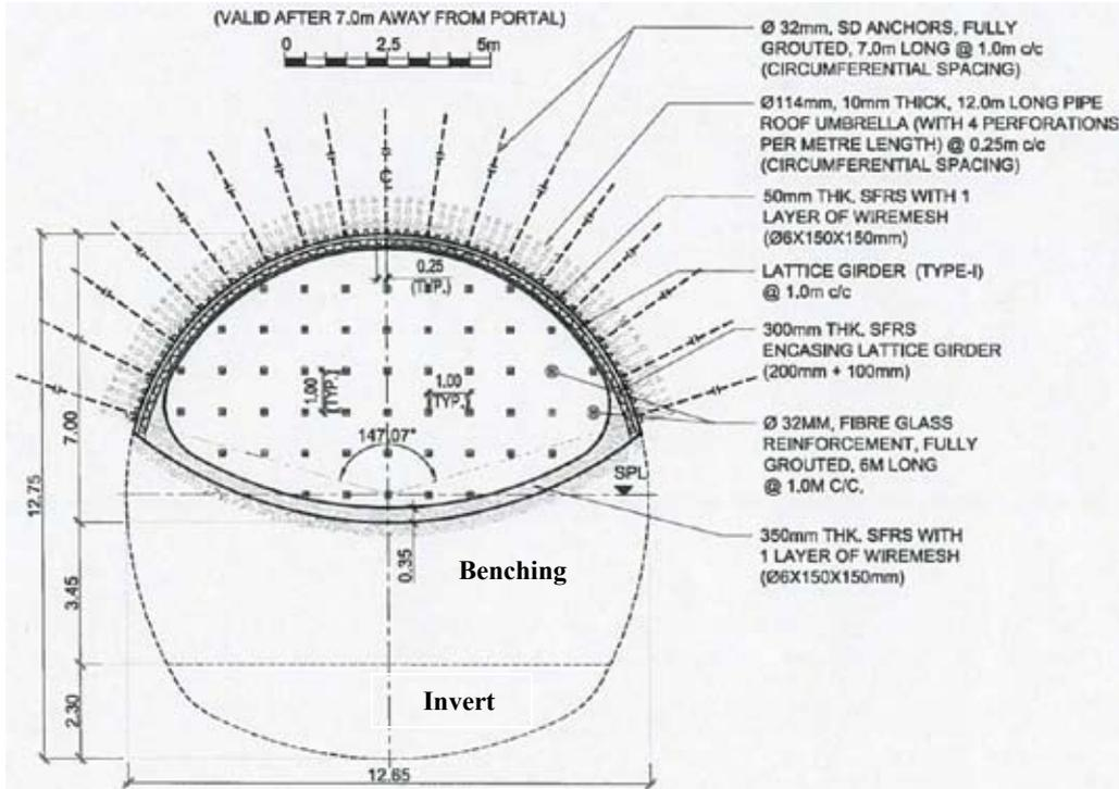
Fig. 4 : Support system for TBM entry Adit
