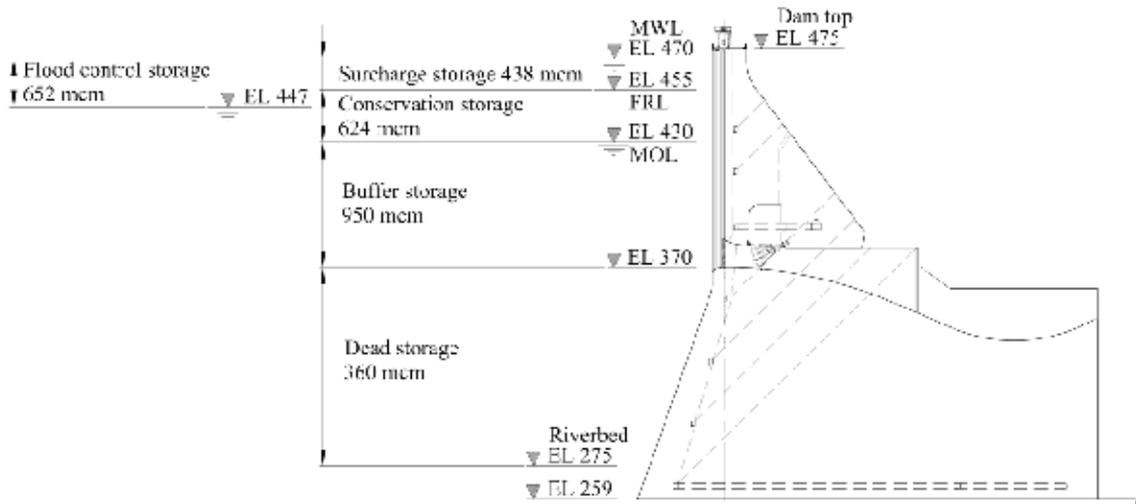
Fig. 2 : Kamala dam spillway section.
