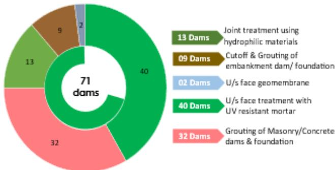
Fig. 13 : Seepage control measures under DRIP.
