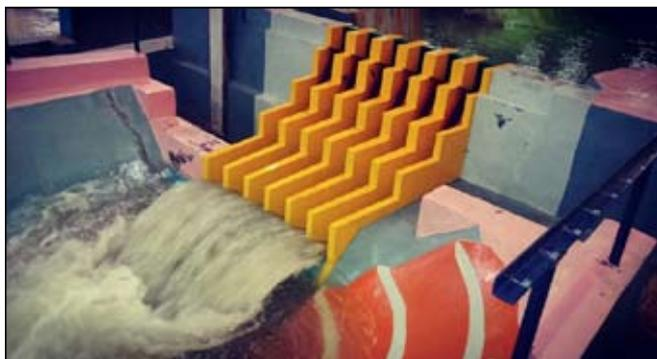
**Photo 10** : Performance of energy dissipator for the discharge of 6500 m<sup>3</sup>/s
