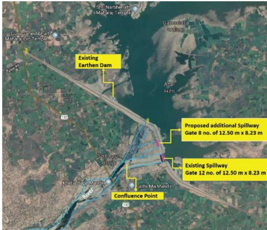
Fig. 12 : Proposed additional spillway
