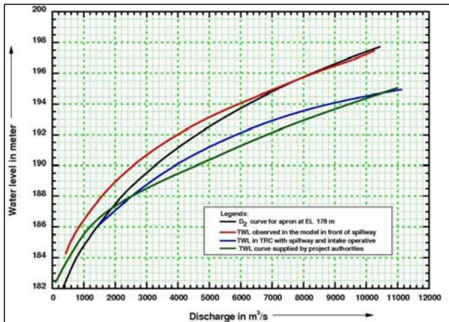
Fig. 7 : Tail Water Rating Curves at 225 m downstream of barrage axis
