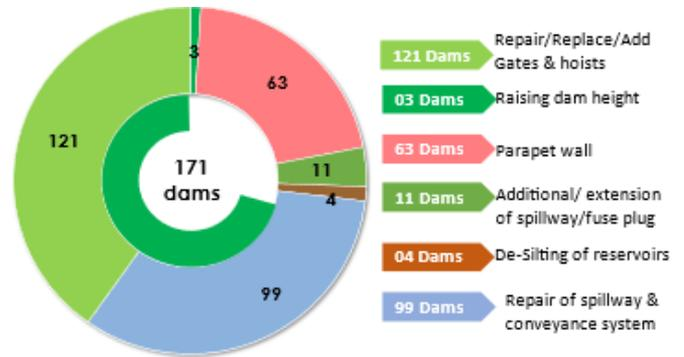
Fig. 5 : Hydraulic safety measures under DRIP.
