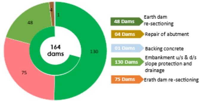
Fig. 10 : Structural safety measures under DRIP.
