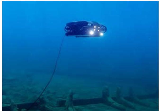
GE Renewable Energy has introduced a new underwater robotized hydropower turbine inspection solution designed to be able to inspect between the runner blades of a turbine – which the company said is a first of its kind in the hydropower condition assessment field. Designed, developed and tested with GE Research Center, the product is based on remote operated vehicles (ROV) equipped with sensors and cameras, and can inspect hard-to-reach areas without dewatering the equipment.
