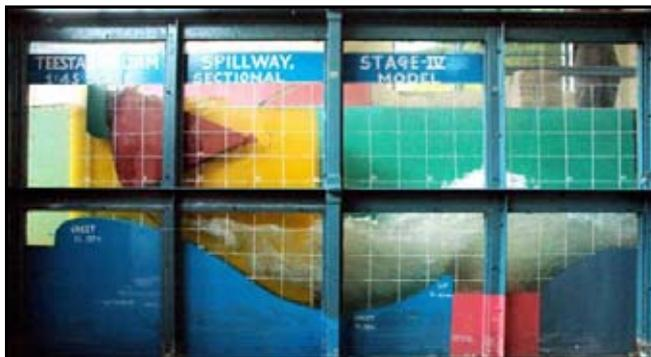
**Photo 13** : Performance of solid roller bucket for gated operation of spillway for the discharge of  $3850 \text{ m}^3/\text{s}$
