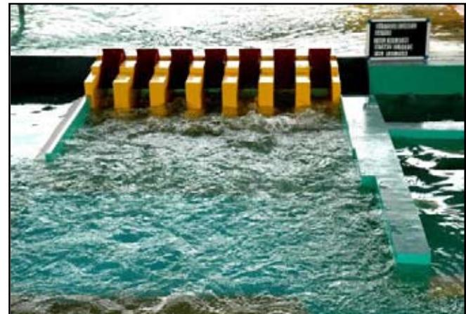
**Photo 15** : Performance of stilling basin for ungated operation of spillway for the discharge of  $7700 \text{ m}^3/\text{s}$
