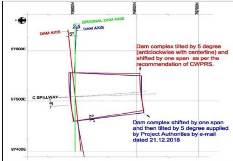
**Fig. 4 :** Superimposed Layout Plan Provided by Project Authorities & Recommended by CWPRS
