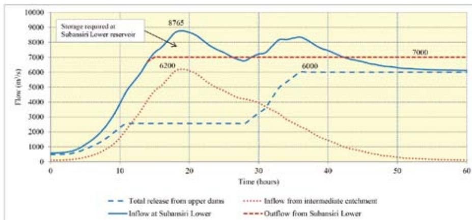
**Fig. 5 :** Flood moderation at Subansiri Lower dam for the regulated outflows from upper dams.
