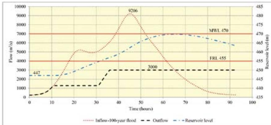
**Fig. 4 :** Routing of 100-year flood hydrograph at Kamala dam
