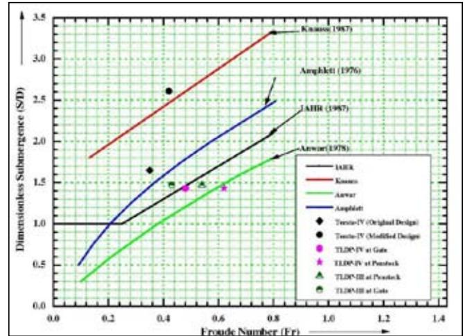
Fig. 2 : Plot of Non-Dimensional Submergence Versus Froude Number
