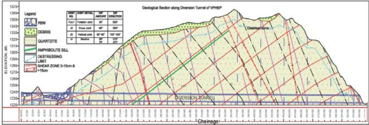
Figure 4 : Geological section along Diversion Tunnel
