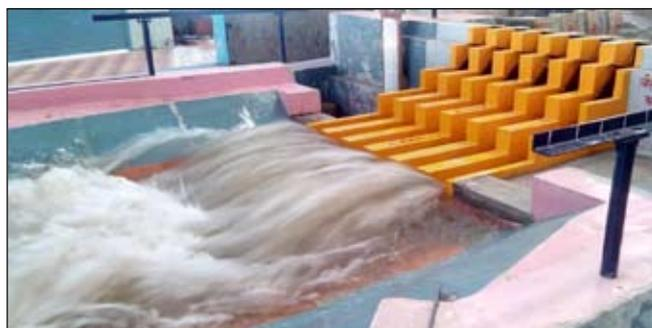
**Photo 3** : Performance of energy dissipator for the discharge of 13000 m<sup>3</sup>/s
