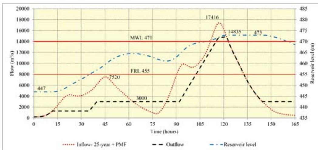
Fig. 6 : Routing of extreme flood hydrograph with one gate inoperative at Kamala dam
