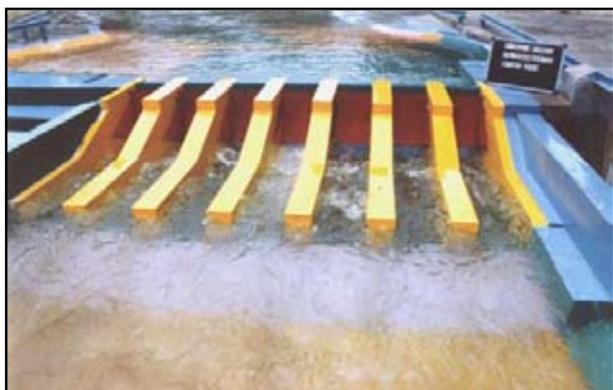
Photo 18 : Performance of stilling basin for the discharge of 7822.5 m<sup>3</sup>/s for gated operation of spillway
