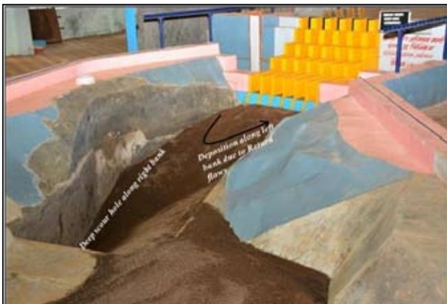
**Photo 7 :** Scour pattern for gated operation of spillway for the discharge of 13000 m<sup>3</sup>/s at FRL El. 755 m
