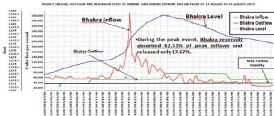
Fig. 16 : Operation of Govind Sagar Reservoir of Bhakra basin during the event of 17th – 18th August 2019
