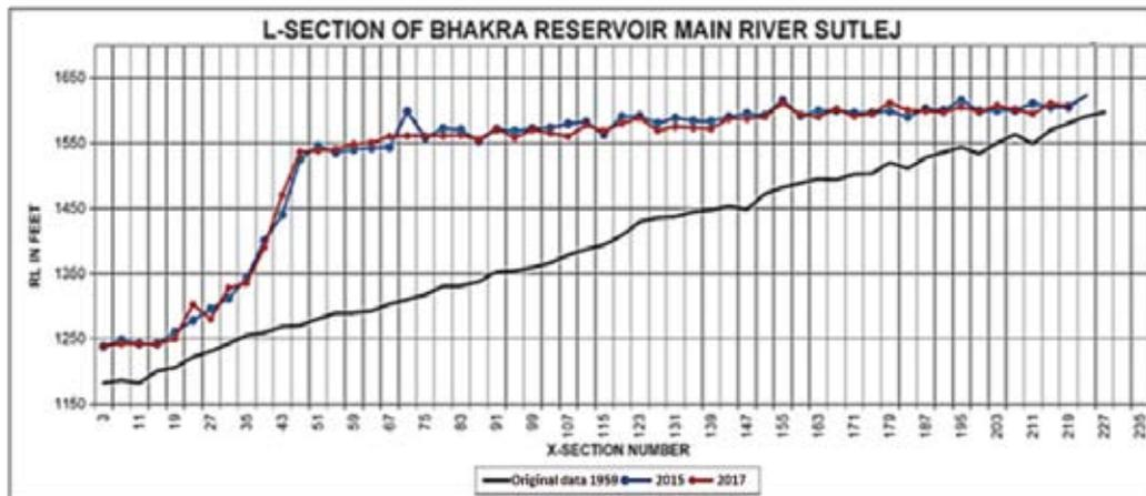
Fig. 9 : L-Section of Gobind Sagar Reservoir
