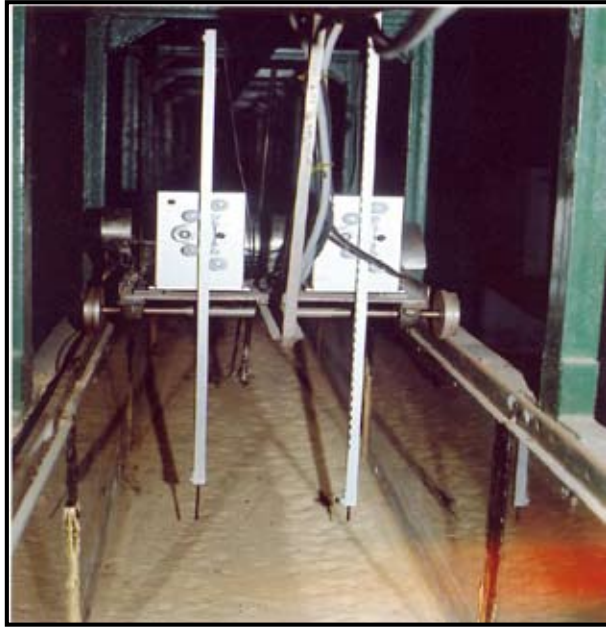
Fig 2 : Photograph of the Bed Profile Indicator (PV-09 System) mounted on the motorized carriage
