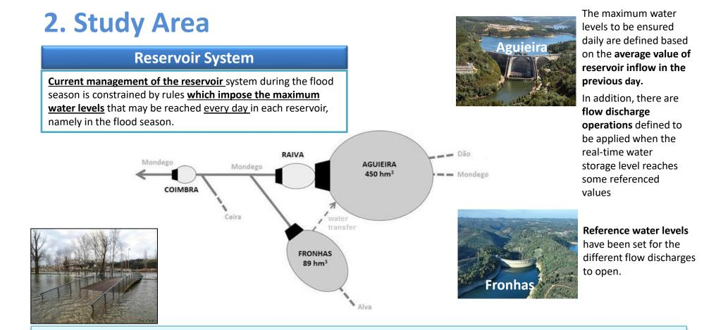
The <u>current operating rules essentially aim</u> at limiting the streamflow to the section of <u>Coimbra</u> to the value of 1200 m<sup>3</sup>/s upon the occurrence of floods with a return period of up to 100 years.
