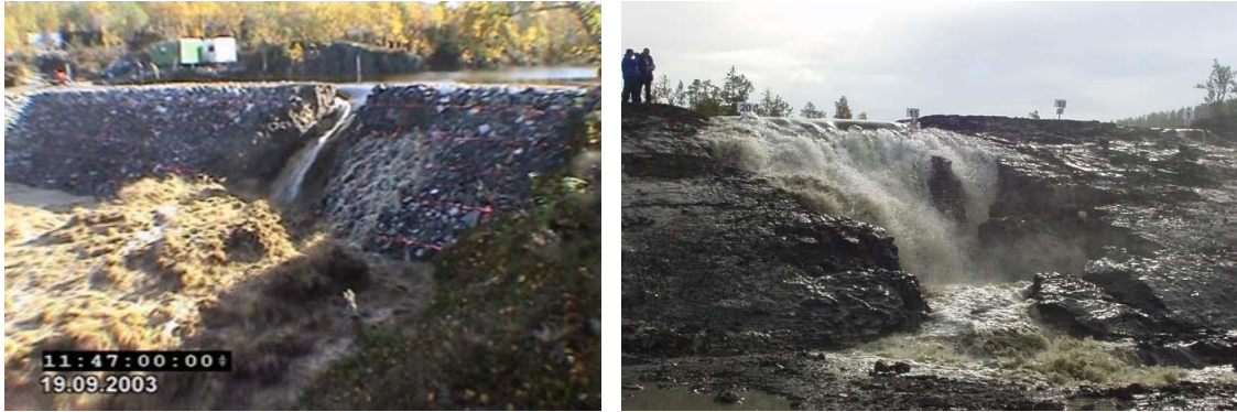
Figure 1. Breach erosion research undertaken through the European IMPACT project.
