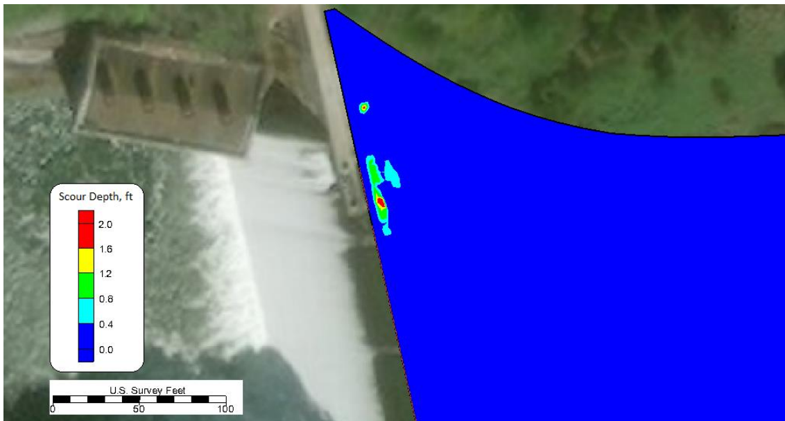
Figure 9. Scour depths near the gate
