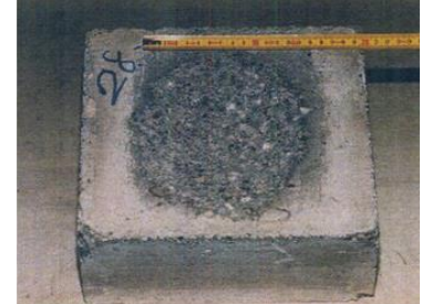
Picture 5: Impact test result on typical B25 concrete
