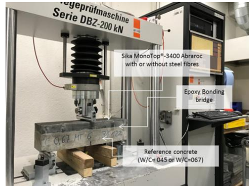
Picture 12: Flexural tensile strength testing of Sika MonoTop®-3400 Abraroc Build-up
