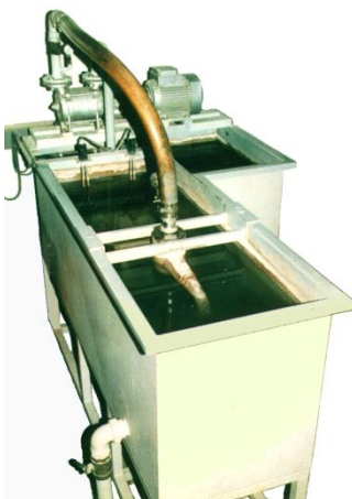
Picture 7: Photo and schematic drawing of the CNT hydraulic abrasion test method
