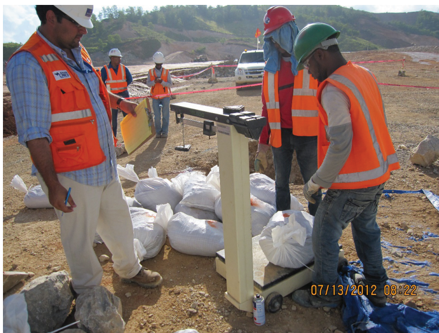
Photograph 6 : The bagged rockfill material weighed by quality control personnel.
