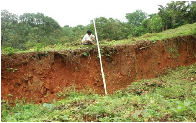
Photo 1 & 2 : Downward slide of overburden soil mass from tension crack.
