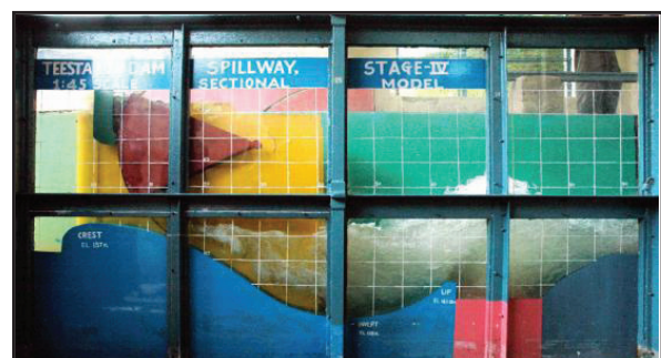
Photo 13 : Performance of solid roller bucket for gated operation of spillway for the discharge of 3850 m 3 /s
