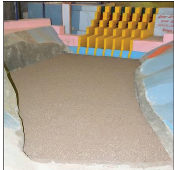
Photo 6 : River bed (scour pit) with erodible bed material in model
