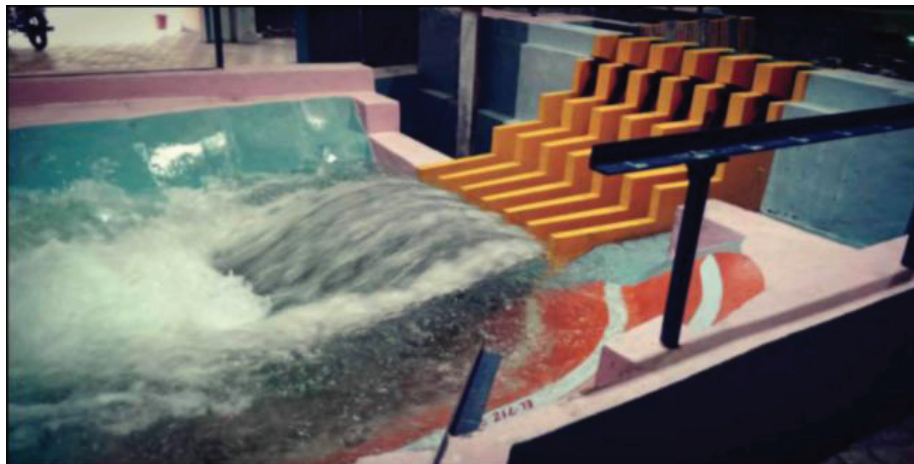
Photo 11 : Performance of energy dissipator for the discharge of 13000 m 3 /s
