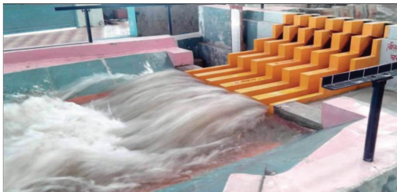
Photo 3 : Performance of energy dissipator for the discharge of 13000 m 3 /s
