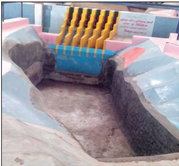
Photo 5 : View of scour pit in model
