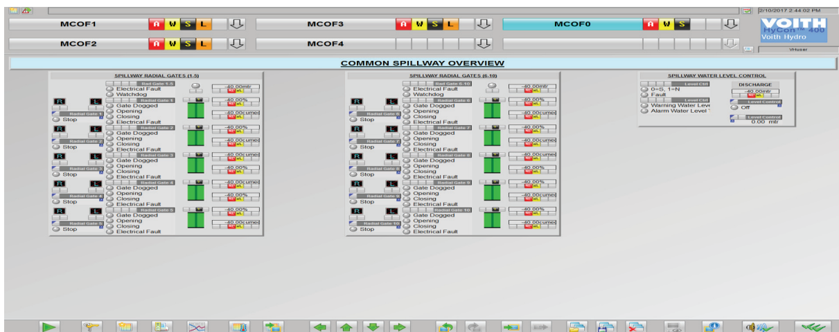
Figure 4 : MCHPP Spillway Structure SCADA Control Overview
