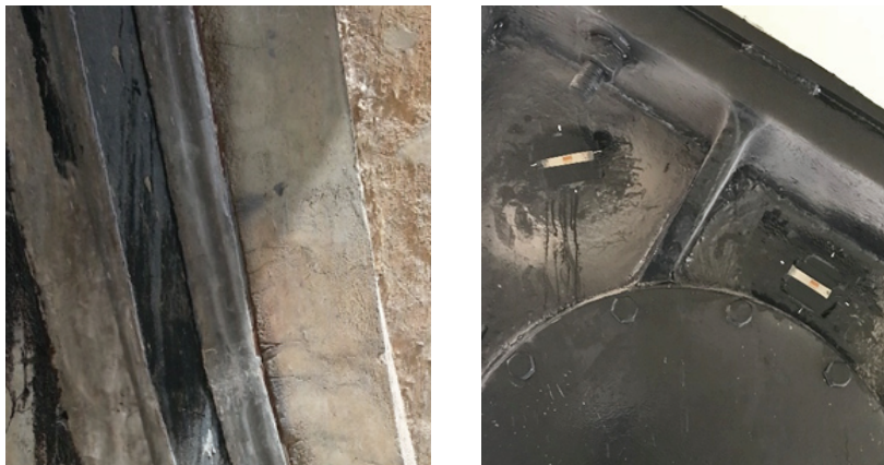
Figure 12 : Roller marks on lateral upper fixed parts (left) and rosettes glued to a trunnion support (right).
