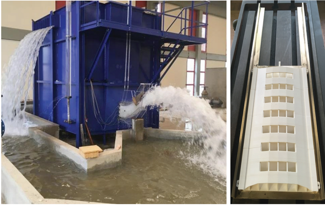
Figure 4 : Physical model. General view on the left and stoplog model (upstream face) on the right.
