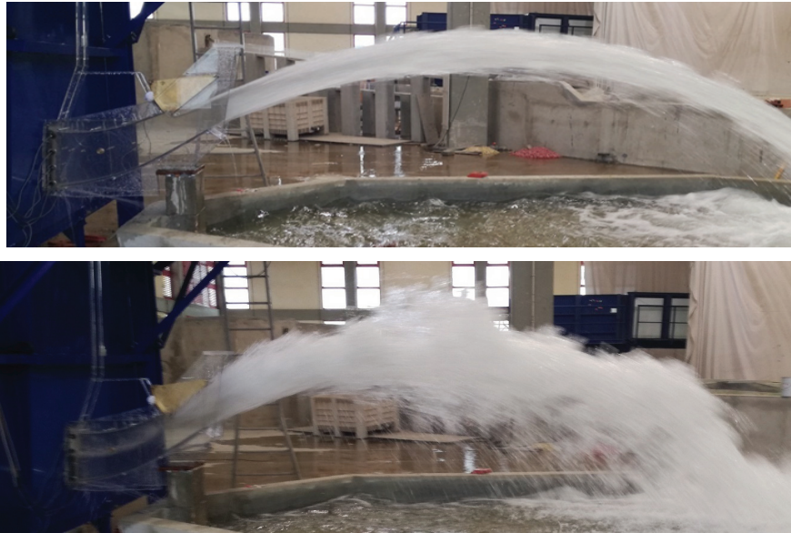
Figure 7 : Jet flow patterns under normal operation (above) and during the stoplog maneuver (bottom).
