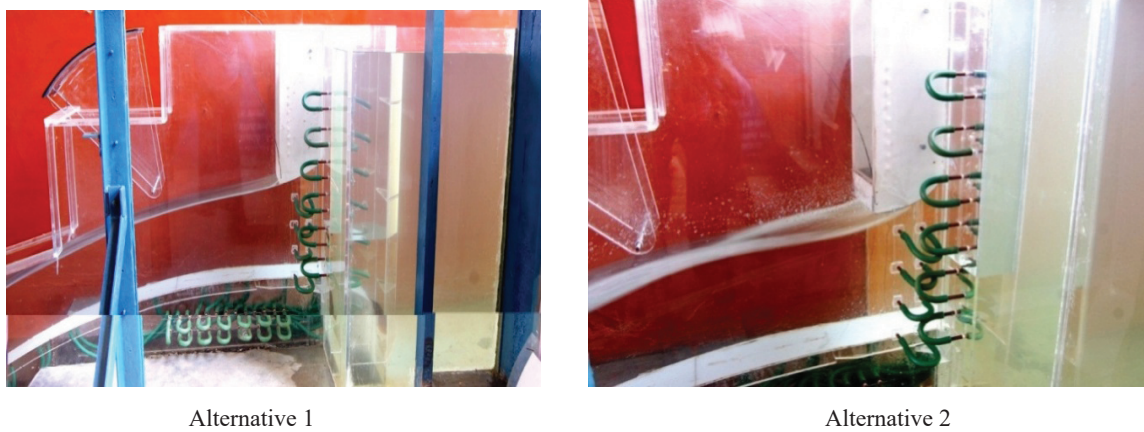
Figure 8 : Flow conditions in the vicinity of breastwall bottom profile for various alternative designs.
