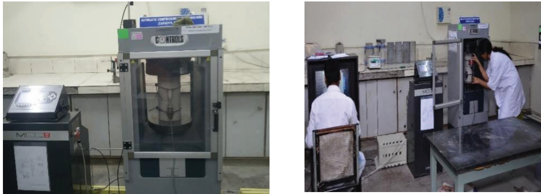
Figure 2 : Test setup for uni-axial compression testing of concrete in Strain Controlled Machine (3000 KN)
