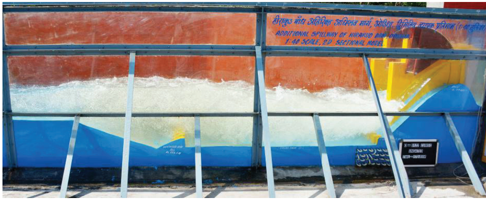
Photo 2 : Flow condition downstream of spillway for ungated operation of spillway for the discharge of 9122 m 3 /s (100%) at RWL El. 191.45 m
