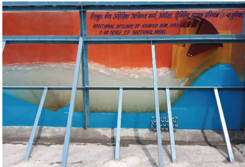
Photo 1 : Performance of stilling basin for gated operation of spillway for the discharge of 6841.5 m 3 /s (75 %) at FRL El. 192.024 m
