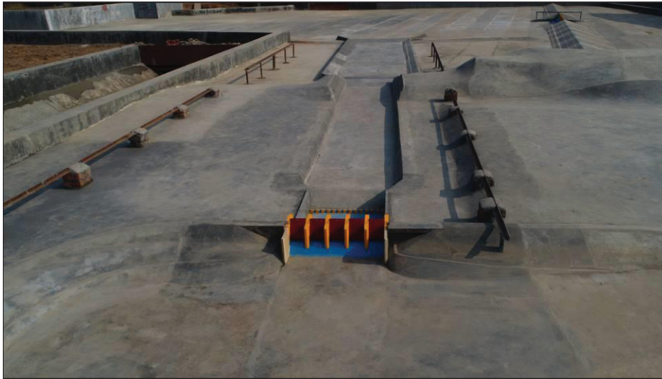
Photo 6 : Side view of the additional spillway model
