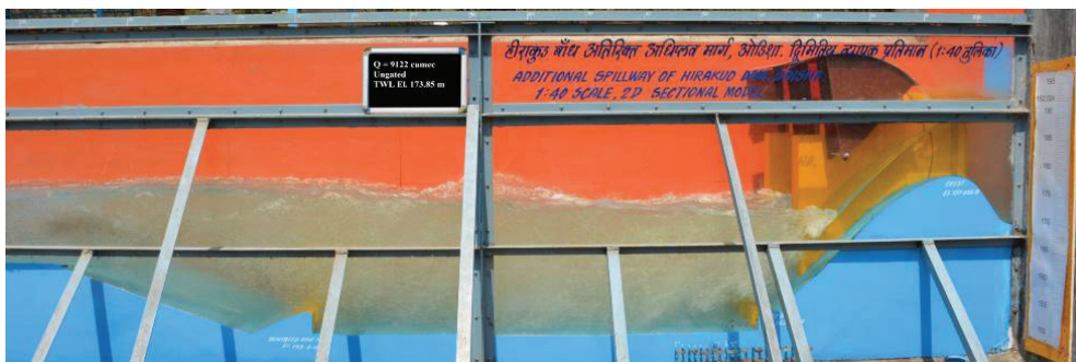
Photo 3 : Performance of stilling basin for ungated operation of spillway for the discharge of 9122 m 3 /s (100%) at FRL El. 192.024 m
