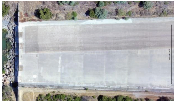
Figure 3 : Example of Optical Imaging of a Spillway Using a Drone
