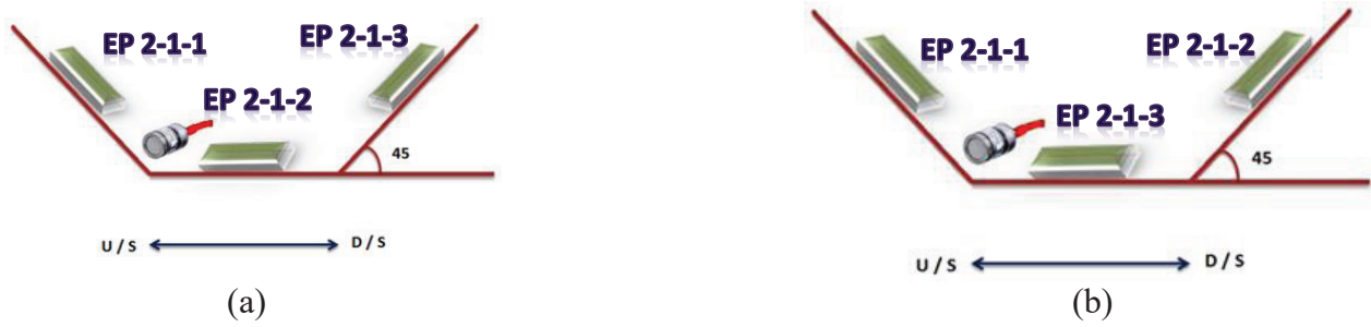
Figure 3 : Position of the stress instruments based on stress petal method, (a) Pattern A, and (b) Pattern B
