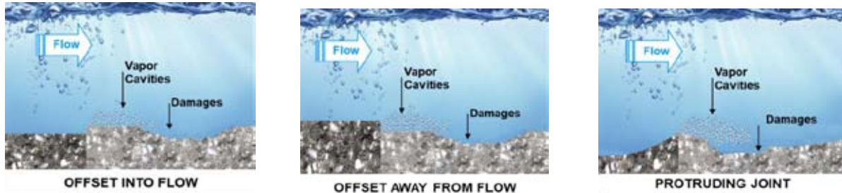
Examples of Cavitation damages @ Surface irregularities
