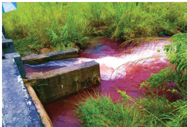
Fig. 6 : Hydraulic connectivity test
