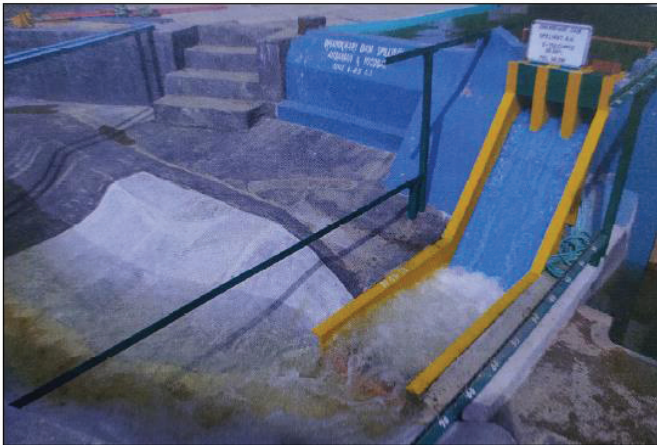
Photo 3 : Flow conditions in model of stilling basin (discharge 150 m 3 /s at FRL)
