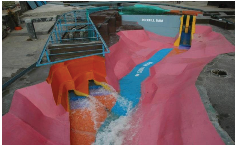
Figure 8 : Flow conditions at the outlet of tunnel spillway
