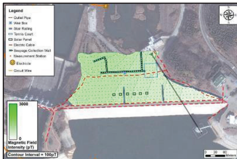
Figure 7 : Expected magnetic field map for homogeneous earth
