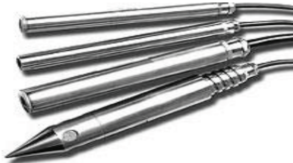
Figure 8. Type of vibration wire piezometer
