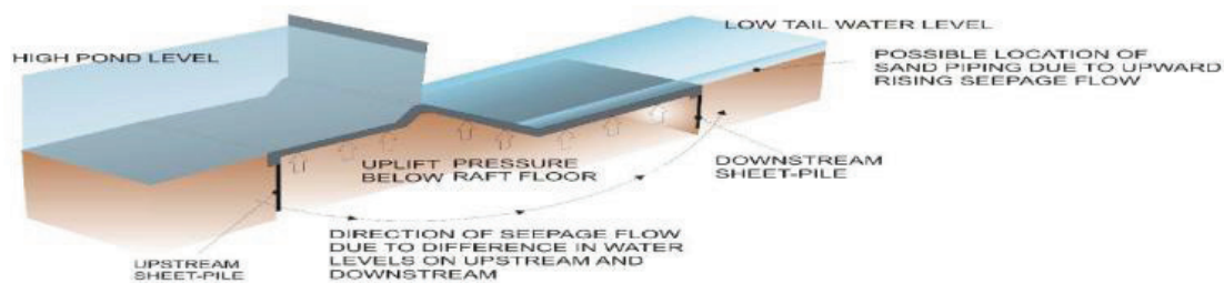
FIGURE 1. Effect of sub-surface flow below barrage floor
