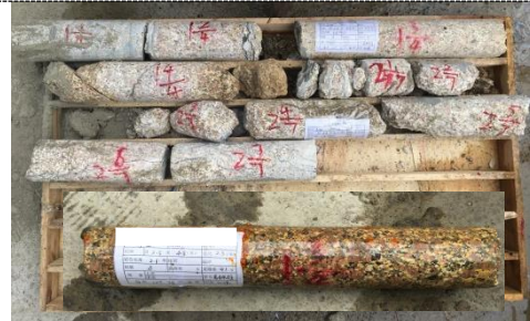
Figure 5. The core samples of post-grouting.
