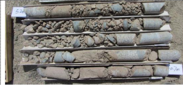
Figure 4. The core samples of dam foundation.
