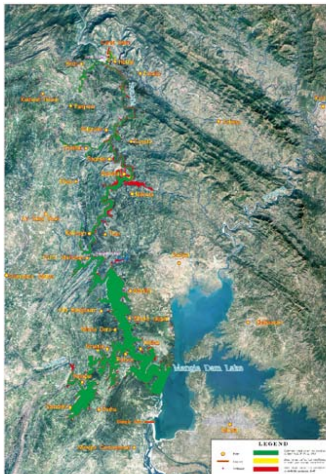
Figure 15. Flooding range map below the Karot hydropower station corresponding to the dam break duration of 2h
