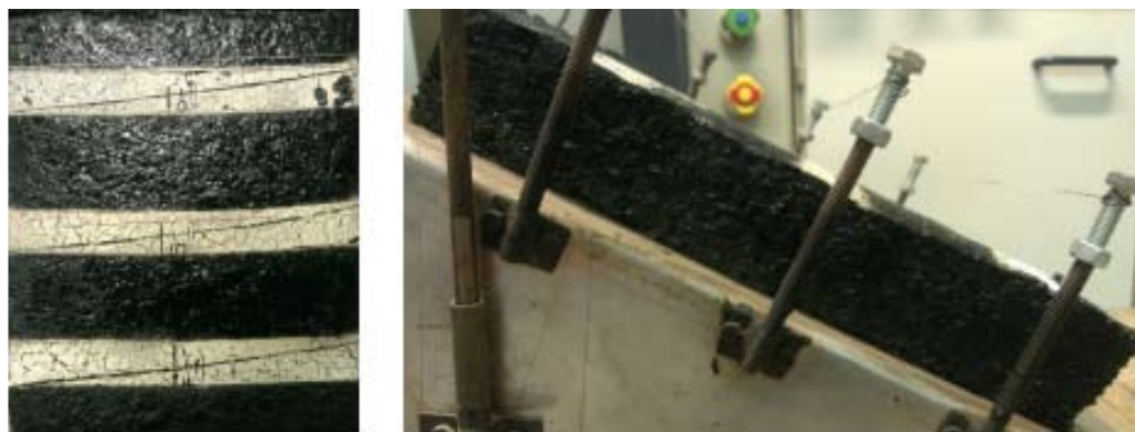
Figure 1 : Dense asphalt produced with LD slag aggregates.
