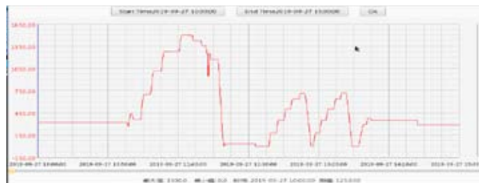
Figure 6 : Showing the discharge hydrograph of the spill way during the vibration test
