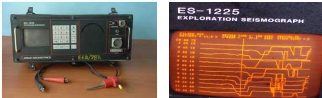
Figure 2 : 12-channel signal enhancement seismograph with accessories and a typical record showing the onset of P-waves at 12 locations
