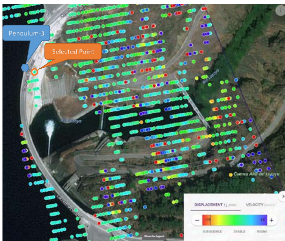
Figure 6 : Displacement comparison between DInSAR and Pendulum in El Atazar Dam
