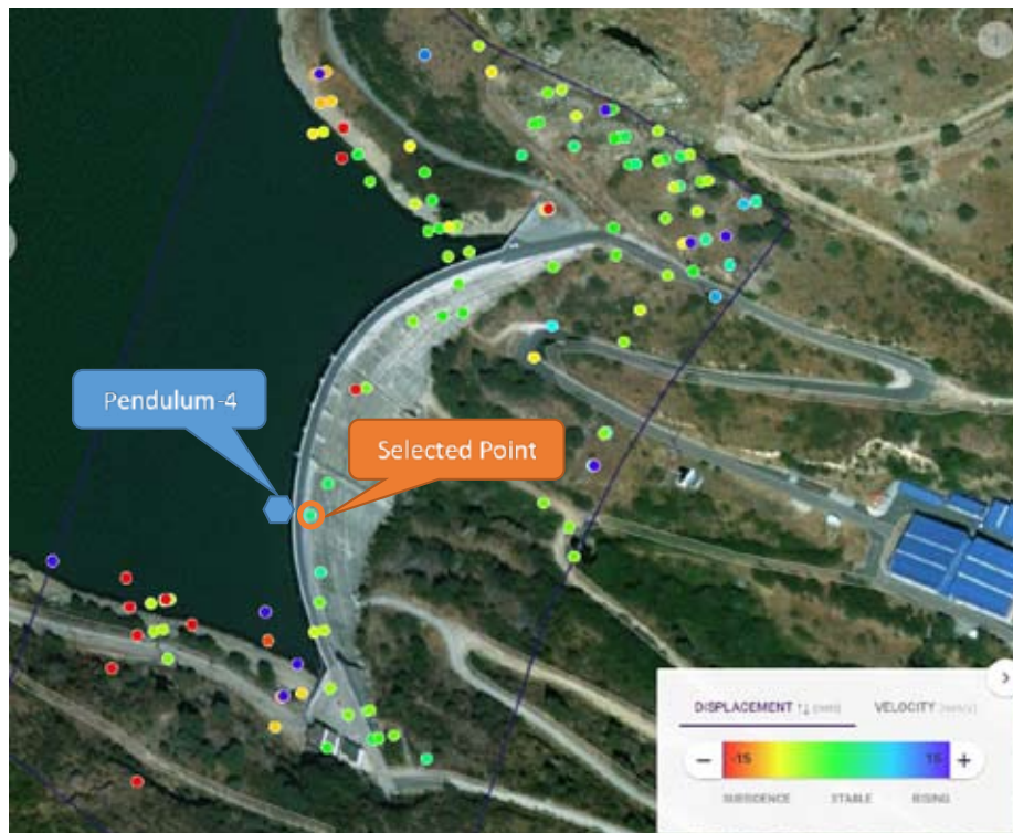
Figure 5 : Displacement comparison between DInSAR and Pendulum in La Aceña Dam
