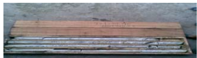
Fig 10 : Good quality core pieces recovered from drill hole DDH-40 having depth of 200m
