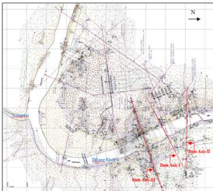
Fig. 1 : Layout Plan of the project area along with location of alternative dam axis.
