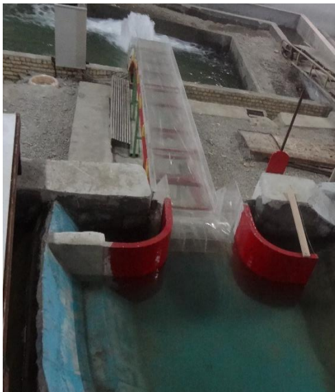
Figure 6: The arc shaped spillway in plan and profile
