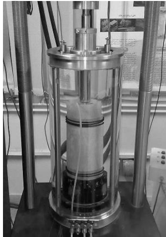
Figure 2. Triaxial cell apparatus during testing
