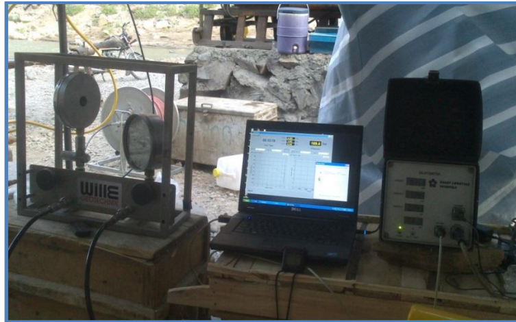
Figure 3. Dilatometer test performance at PD1 borehole in river bed at GhezelOzen (Pirtaghi) Dam site
