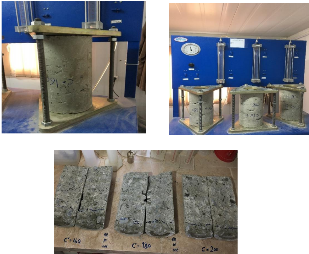
Figure 6- Performing Water Influence Depth Test of Rcc Mixing Plans with All In One Materials
