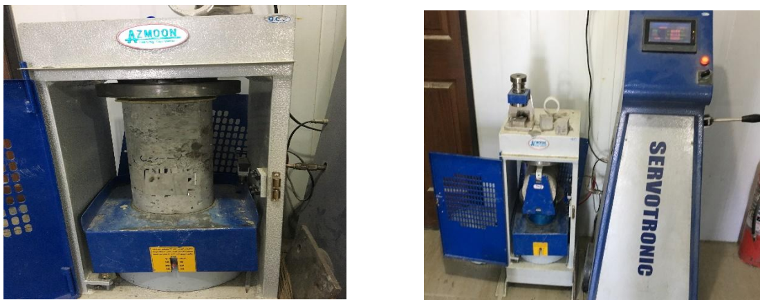
Figure 7-Tests to determine compressive strength and tensile strength of Rcc mixing designs with All In One.
