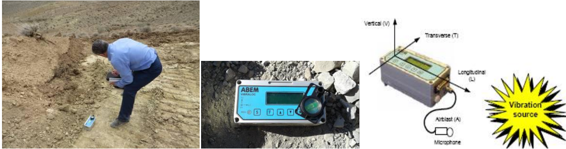
Figure 4. digital seismograph/ Installation and arrangement
