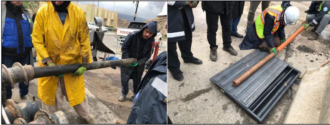
Figure 8 Clay core log using continuous core method.
